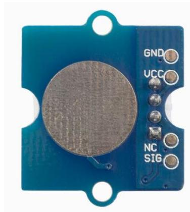
Grove - Touch Sensor enables you to replace press with touch. It can detect the change in capacitance when a finger is nearby. That means no matter your finger directly touches the pad or just stays close to the pad, Grove - Touch Sensor would outputs HIGH also.
