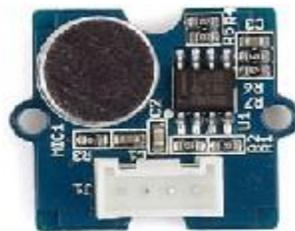
Grove - Sound Sensor can detect the sound intensity of the environment. The main component of the module is a simple microphone, which is based on the L358 amplifier and an electret microphone. This module's output is analog and can be easily sampled and tested by an Arduino.
